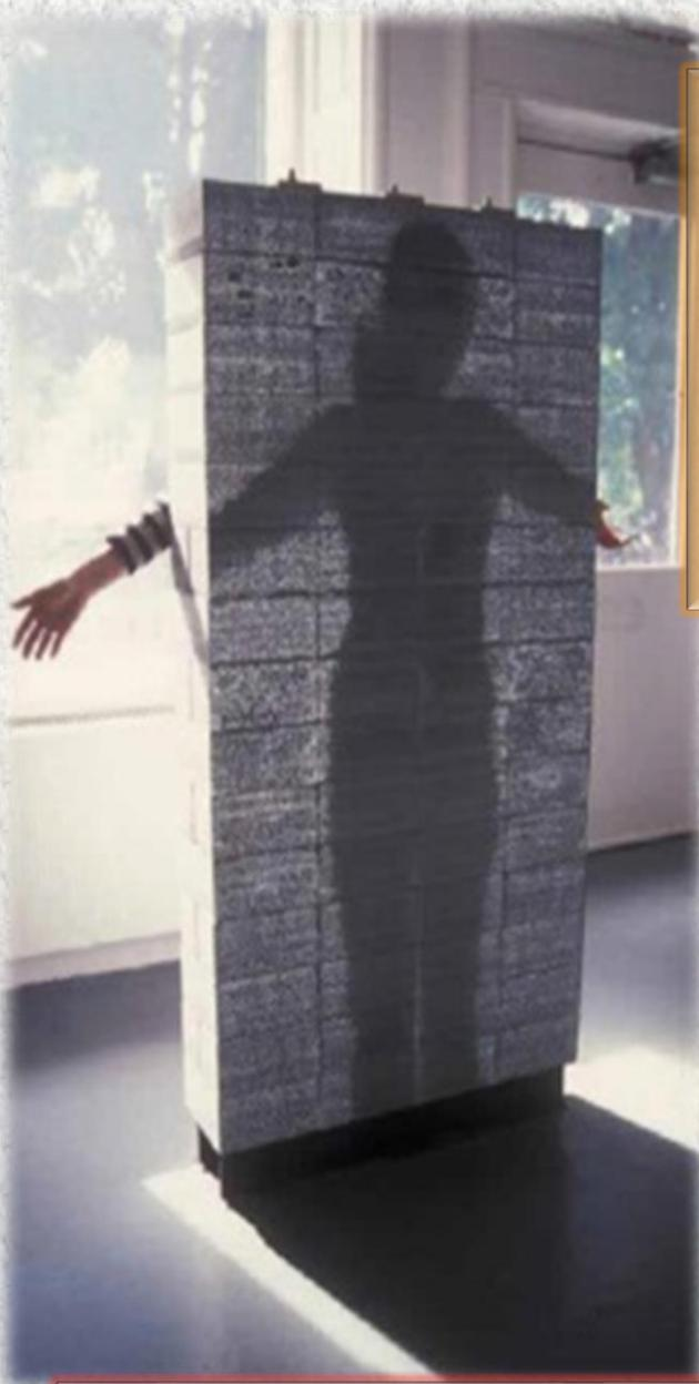
LiTraCon is a light transmitting concrete building material developed in 2001 by Áron LOSONCZI and his team.
